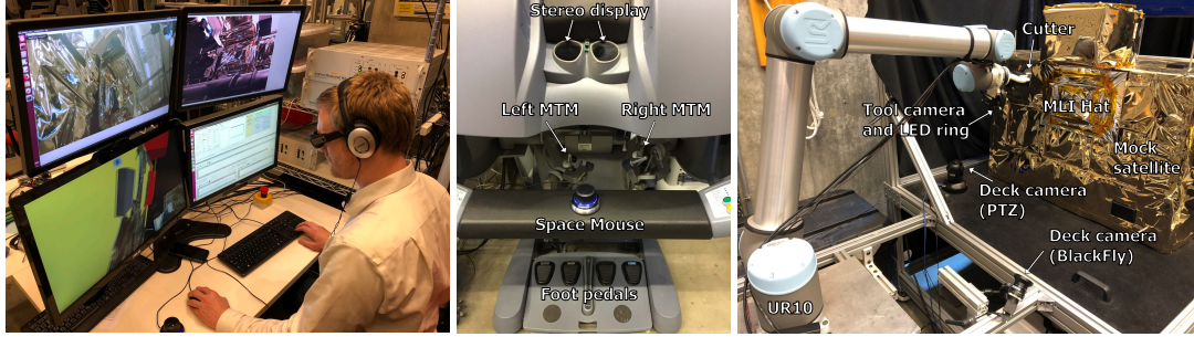
Figure 3.2: Left: Conventional teleoperation keyboard and GUI (KB); Center: da Vinci master console (dV) with space mouse; Right: remote robot with satellite (see Fig. 3.3 for closeup of cutting assembly). Left image shows operator performing trial with augmented virtuality (AV) visualization on 3D monitor (lower left monitor). Operator is wearing noise-canceling headphones and 3D shutter glasses. Conventional (CAM) visualization is similar, except that lower left monitor shows 2D camera image. Lower right monitor shows robot control GUI (also shown in Fig. 3.5).
