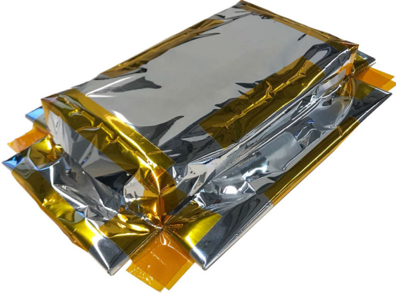
Fig. 7. Realistic mock-up of MLI “hat.”
